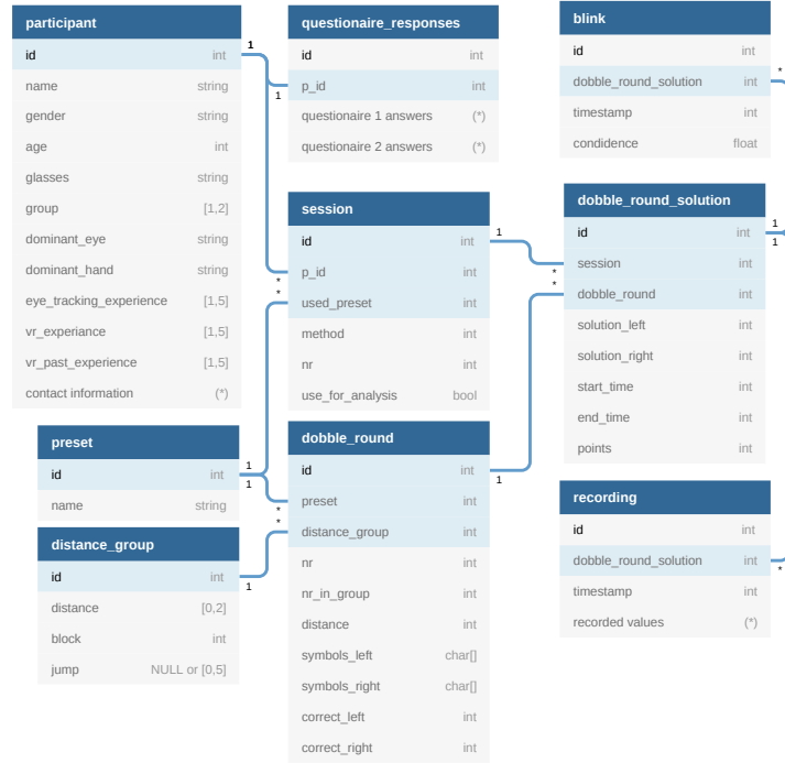
Figure 5.3.: Database schema used to save experiment design and recording. Fields marked with (*) include multiple fields in the real database that were omitted here for simplicity. Recorded values can be found in section 5.5; Questionnaire questions can be found in section 5.6.
